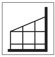
Use minimum expansion space of  $\frac{1}{2}$ ". Climate conditions should be between 55° & 85° F and 30 to 55% relative humidity 48 hours prior to, during the duration of the installation and 48 hours after the installation is completed.
