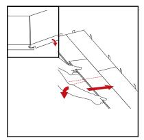
At a slight angle, insert tongue end into the grove end of the previous plank. Get as close to the side of the previous plank as possible. Also at a slight angle, press the side tongue into the groove of the plank next to it. Press gently to engage the planks.
