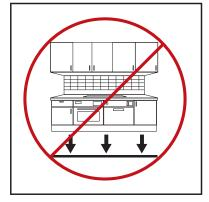
Installation of built in cabinets inhibits the ability for the floor to expand and contract. Perimeter gluing is also not recommended for the same reason.
