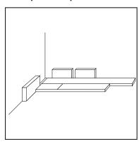
Standard expansion space should be factored at ¼" and this will suffice for a floor that does not exceed 50' in span or width.
