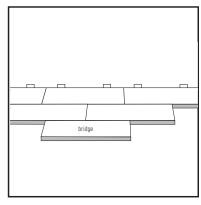
Using a cut piece of approximately 12" to 14" in length, form a temporary bridge next to the end of the plank just installed.
