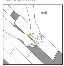
The last row of planks may need to be cut widthwise to achieve the correct width. The width of the last row must not be less than 2". This is accomplished by measuring the room prior to installation and factoring how many rows it will take to complete room.
