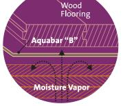
Aquabar "B" helps slow moisture vapor originating below the wood floor system.
