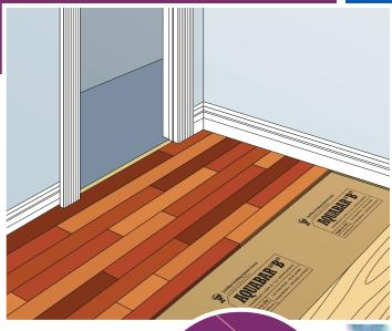
Aquabar "B" hardwood floor and tile underlayment is an extremely effective moisture vapor retarder for use in a variety of interior construction applications. Consisting of two layers of kraft paper laminated with asphalt, Aquabar "B" is a nono-reinforced 30/30/30 duplex type Grade "B" paper.
