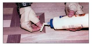
• **Step 2:** Apply wood glue to one side of the sliver. Use the appropriate glue such as PVA. The glue must be strong enough to hold the sliver during the sanding process.
