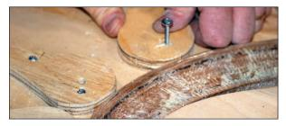
Continue installing the cams, wedges or clamps. Pressure applied by the cams, wedges or clamps should pull the laminations toward the end of the assembly, rather than pushing the laminations toward the middle. Use as many cams, wedges or clamps as possible.
