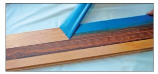
• **Step 8:** Once the tint is completely dried, apply another coat of finish. Remove the tape before the finish dries (remember to pull the tape away at the correct angle).
