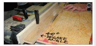
• **Step 5:** Set the blade on a 7-degree angle and adjust its distance from the fence for the width of the board.
